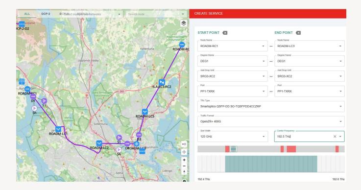
After a service is configured, the information is stored in the SoSmart Controller database. All provisioned services can be viewed in a detailed service list in a separate window or in a miniature list in the network window.
